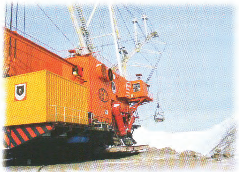
Dragline ESH 90/15 - main hoist drive equipped with electrohydraulic disc brakes operated by ELHY ® - thrusters
