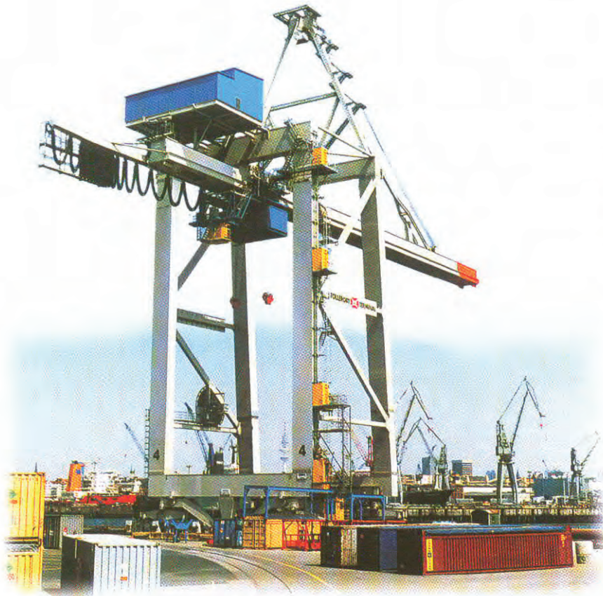
KBE Gernsheim, double-link level luffing crane with 14 ELHY® units
