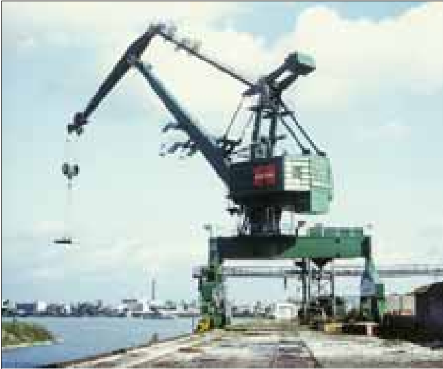
KBE Gernsheim, double-link level luffing crane with 14 ELHY units
