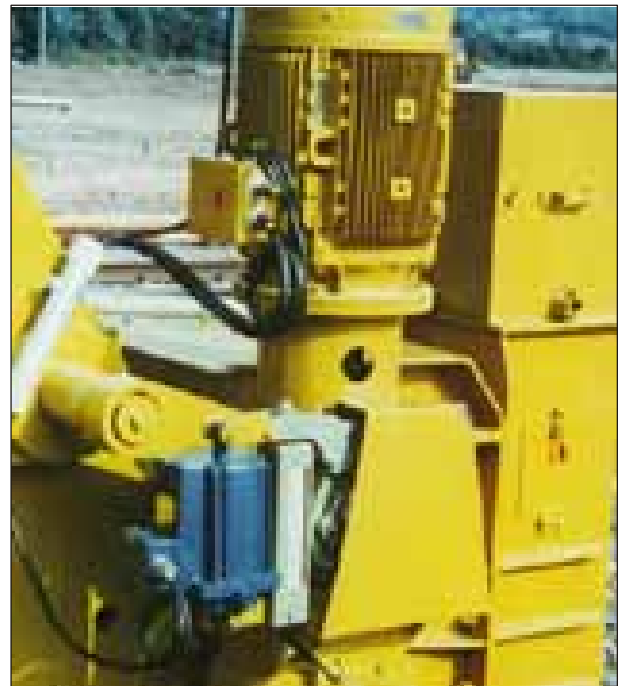
Kranbau Eberswalde, balancing crane 6 t x 40 m equipped with 4 ELHY units EB 220 – 50/2 (at YBBS, Austria)
